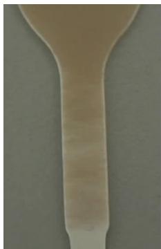
Fig. 6 The photo of initial stretching stage of PLLA/NBR system
